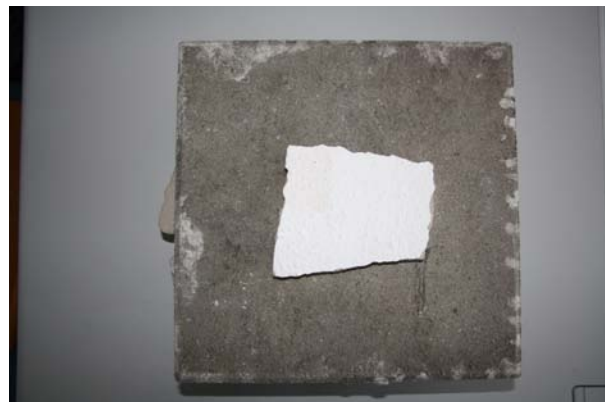
Fig. 2: photo of the test specimen consisting of a single plaster piece applied to a concrete plate (top view)
